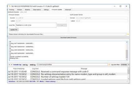
4. Connect again to the Swift Console and go to the Firmware Update tab. Verify the firmware version.
