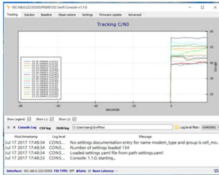
2. Go to the Firmware Upgrade tab, Select the Binary File to be uploaded into Piksi Multi and click Upgrade FW.
